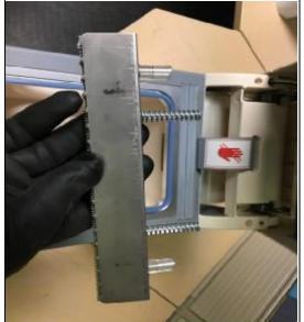
Make sure to remove all broken parts in case of plastic knife seat is broken.
