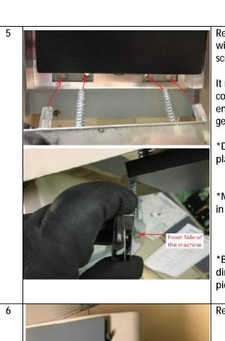
Replace the broken assembly with the new one. You will need to hold the new assembly in place while screwing in the 2 screws.
