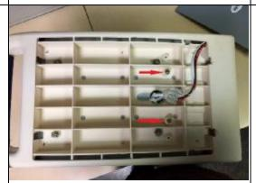
You will now see a couple of screws when you remove the lid on the top side of the hood. Unscrew the 2 screws as shown on the picture with a Philips screw driver while holding the knife assembly from the other side. Use protective gloves to hold the knife assembly.
